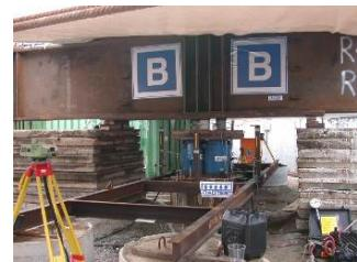
Pile head with additional reaction beam
